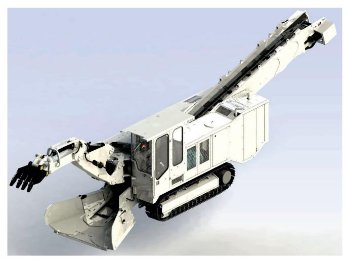
For heading in soft ground and high speed mucking of blasted rock
