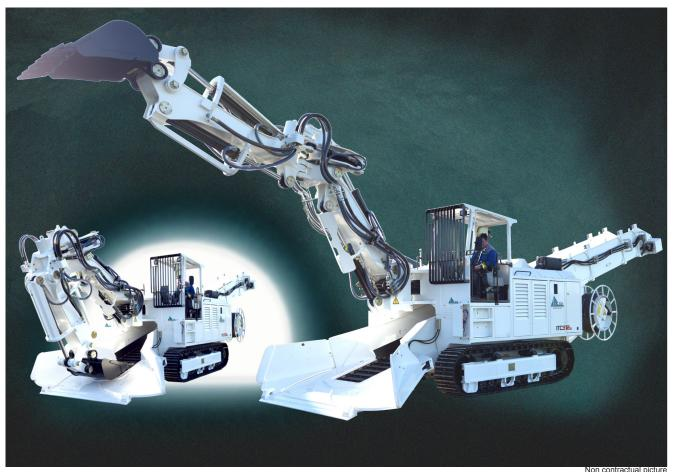
Excavation boom with swivel dipper stick for heading in soft ground
