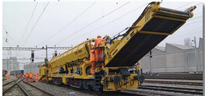
Reduced space requirement thanks to onboard conveyor
