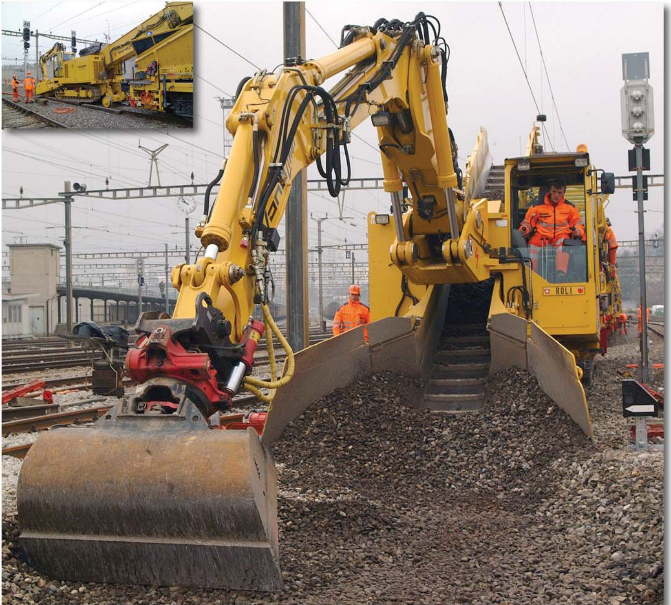
The ballast loading machine Schaeff model ITC 312 VL2 with jointed boom in loading position
