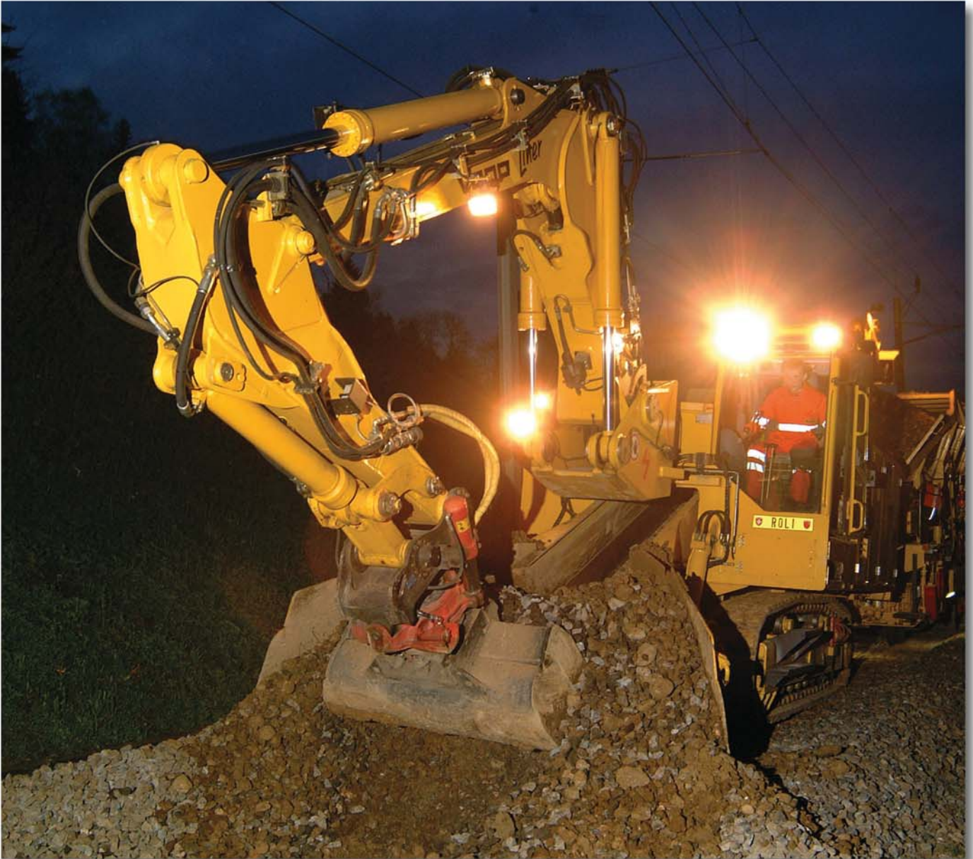
The ballast loading machine Schaeff model ITC 312 VL2 with jointed boom in loading position
