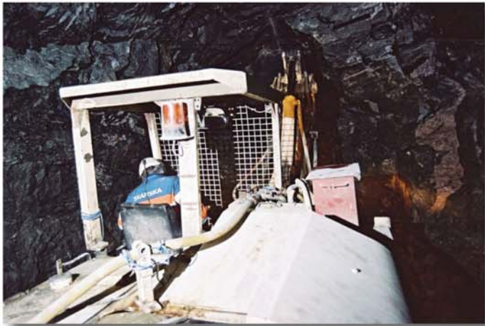
Picture 5: FOPS cab with grid for safe scaling
