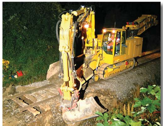
Acurate working thanks to the Roto-Tilt device
