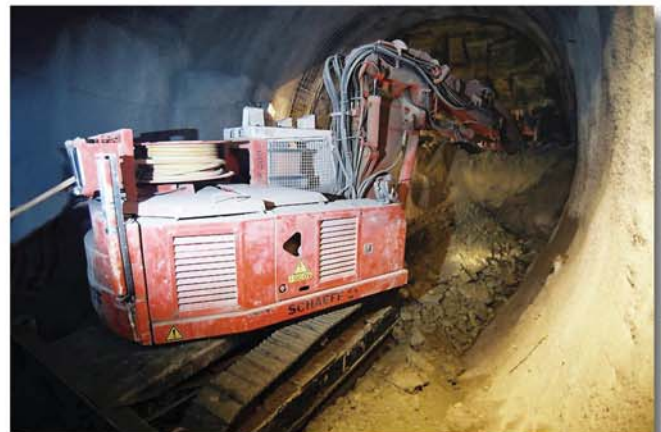
The cable reel is located on the upper carriage
