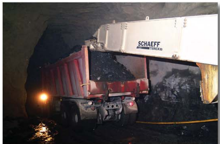
The loading machine ITC 312 while loading onto 18 m 3 trucks
