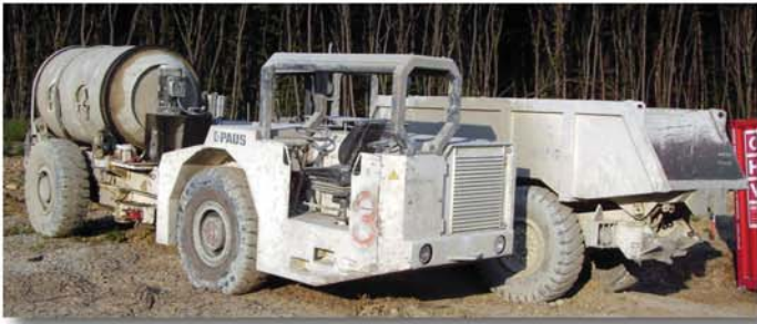
The Dump truck with a concrete mixer drum
