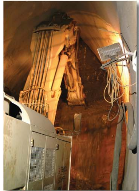
The compact Tunnel Heading Machine Schaeff model ITC 112 M4
