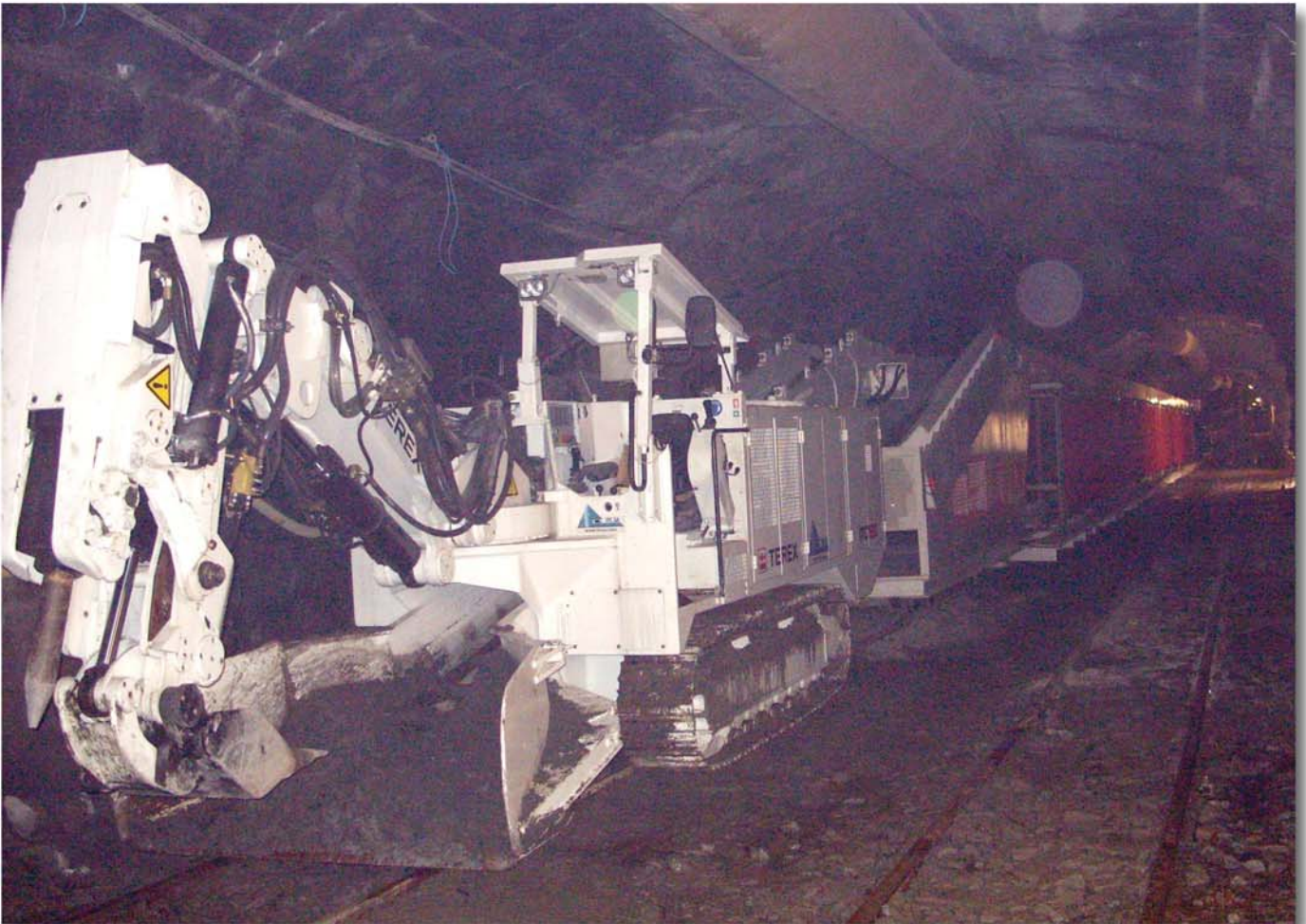
The Tunnel loading machine ITC 120 F6 in composition with the backup
