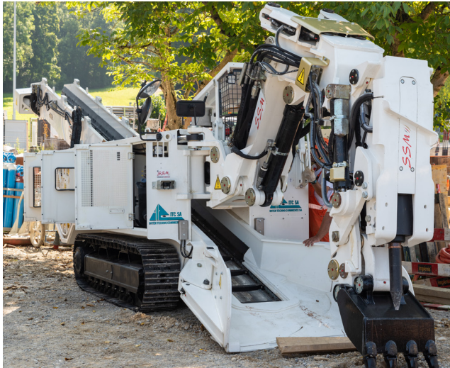
The 14.5m 2 section is narrow, but the ITC125 will work through it without any problems.
