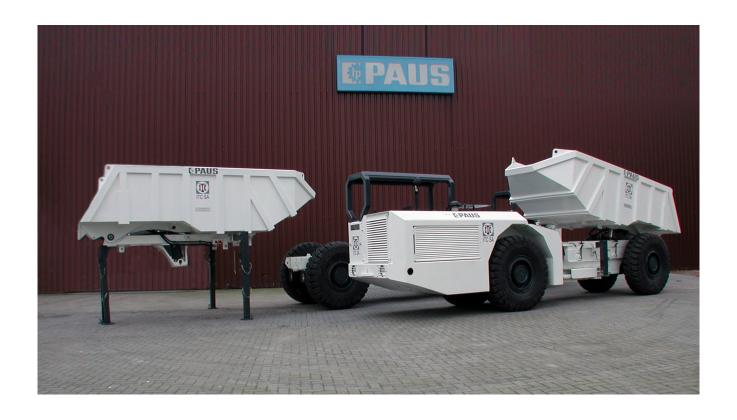
Tunnel articulated Dump Truck PAUS model ITC 10000A with all wheel drive and reverse seat for interchangeable structures
