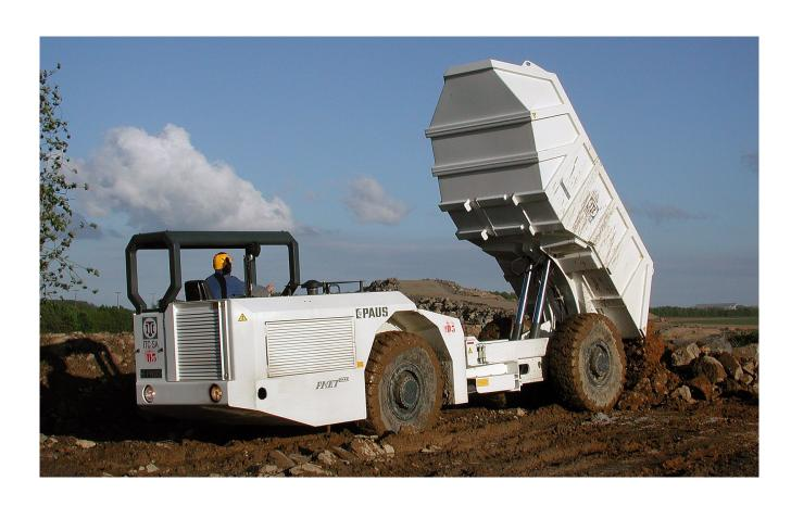
Tunnel articulated Dump Truck PAUS model ITC 10000 with all wheel drive and reverse seat
