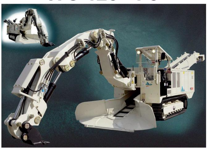
For heading in soft ground, for scaling and high speed mucking of blasted rock
