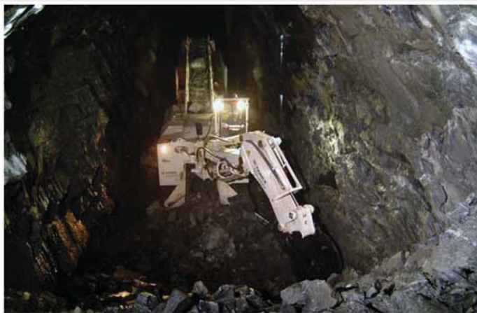
The Superloader ITC 312SL while mucking at high speed
