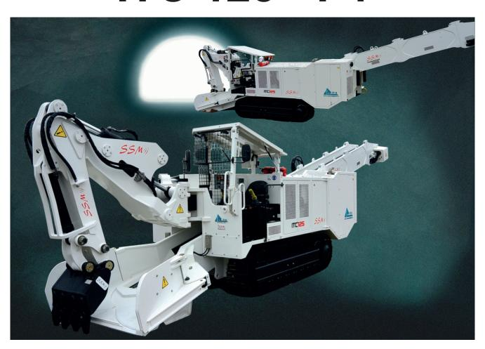
For heading in soft ground and high speed mucking of blasted rock
